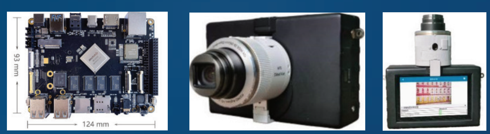
Figure 4. RK3399 Core Motherboard and Implementation of Embedded Handheld Terminal
